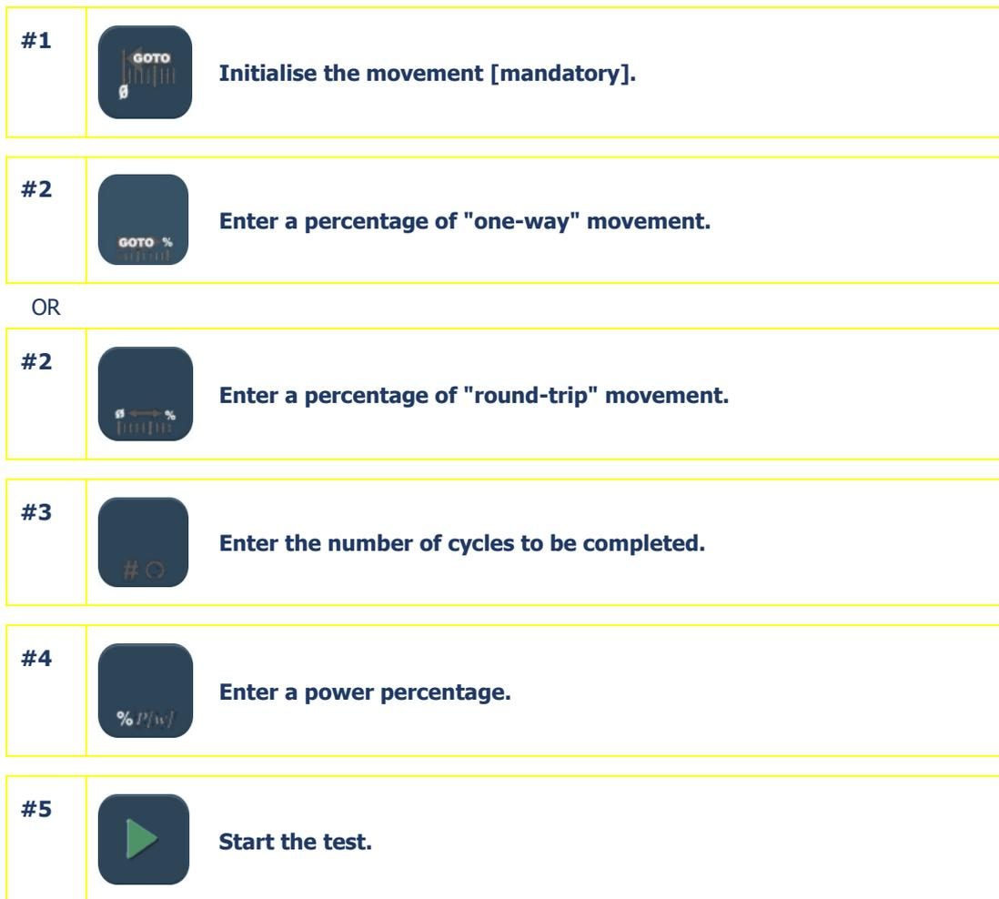
Flow chart 6-1: Operating principle of a typical test screen
