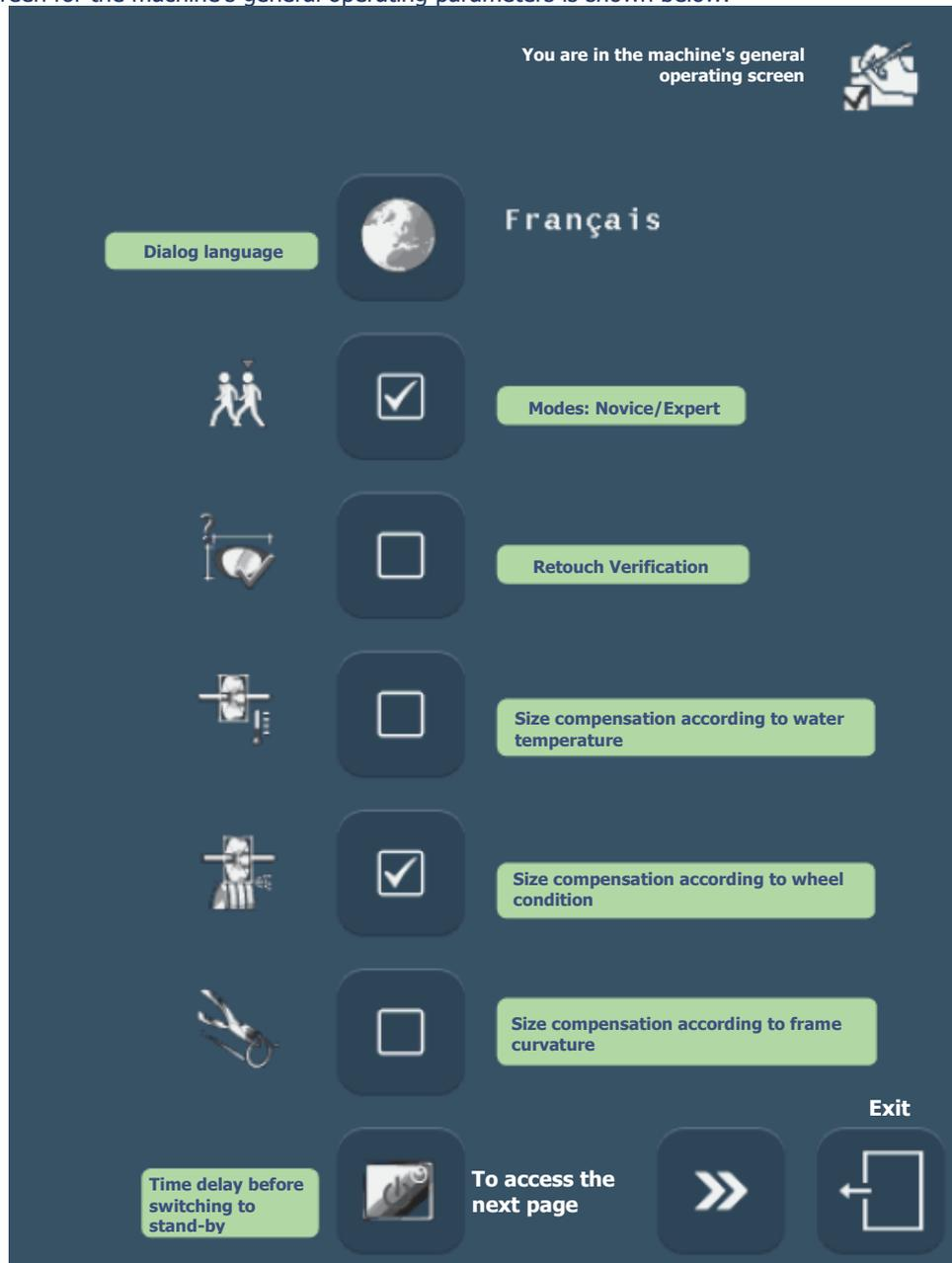
Screen 4-8: Setting the parameters of the machine's general operating functions (Page 1)
