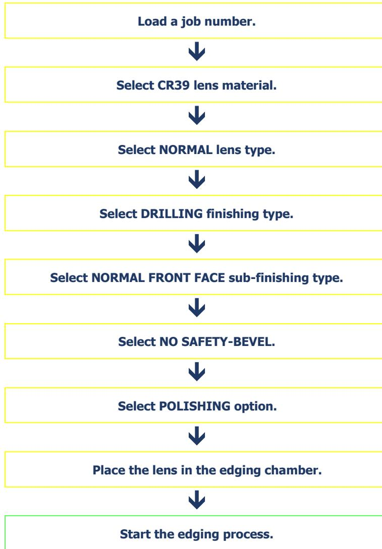
Flow chart 3-6: Production of a job with Drilling finishing
