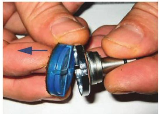
Illustration 5-1 : Replacing the flexible lens clamp adaptor pad
