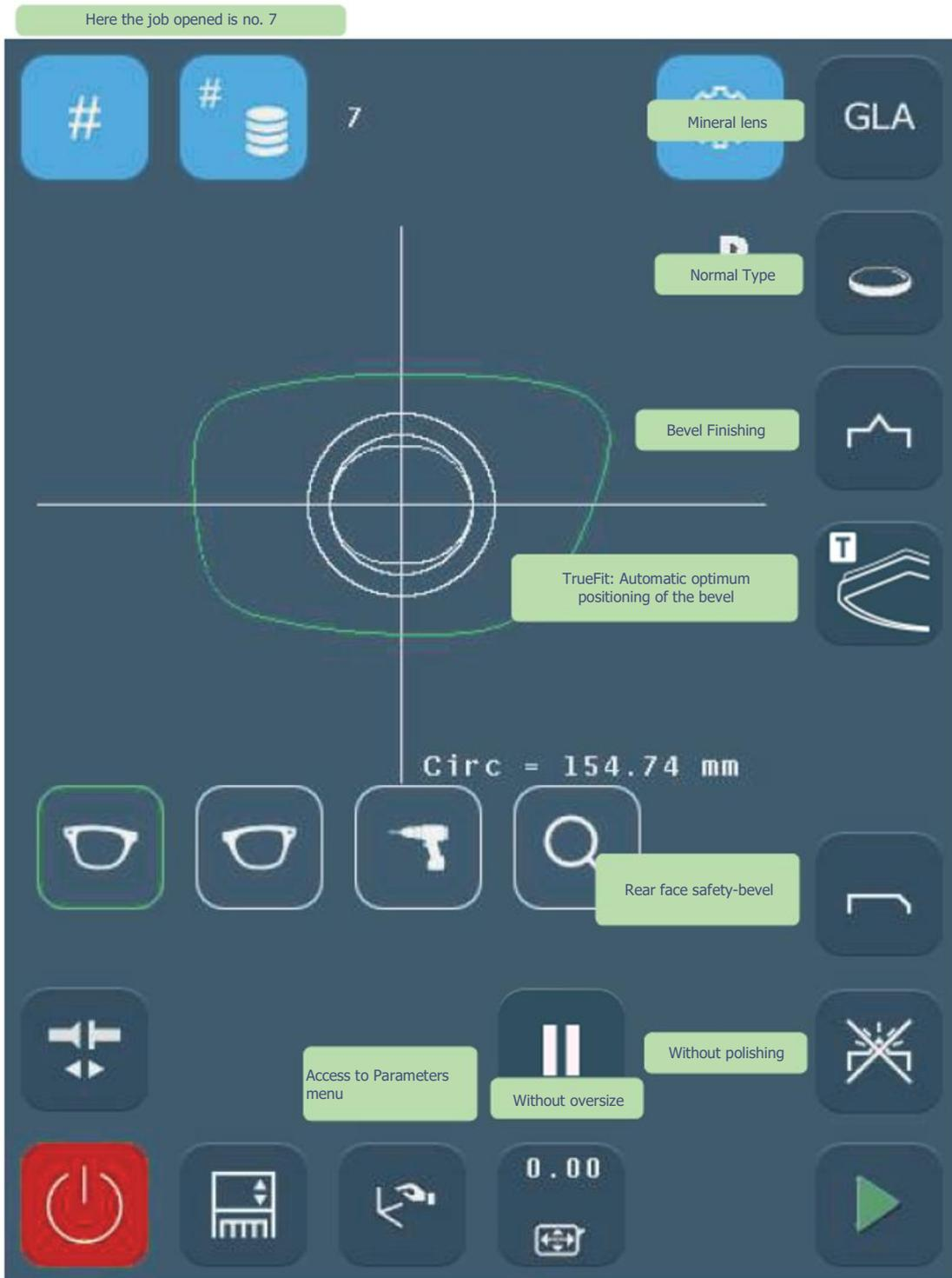
Screen 3-20: Example of the production of a job with a bevel
