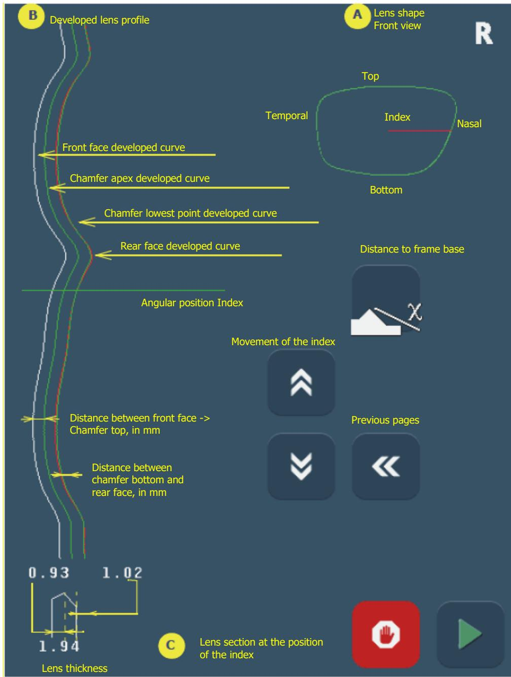
Screen 3-32: Control screen of chamfer at frame base (page 3)
