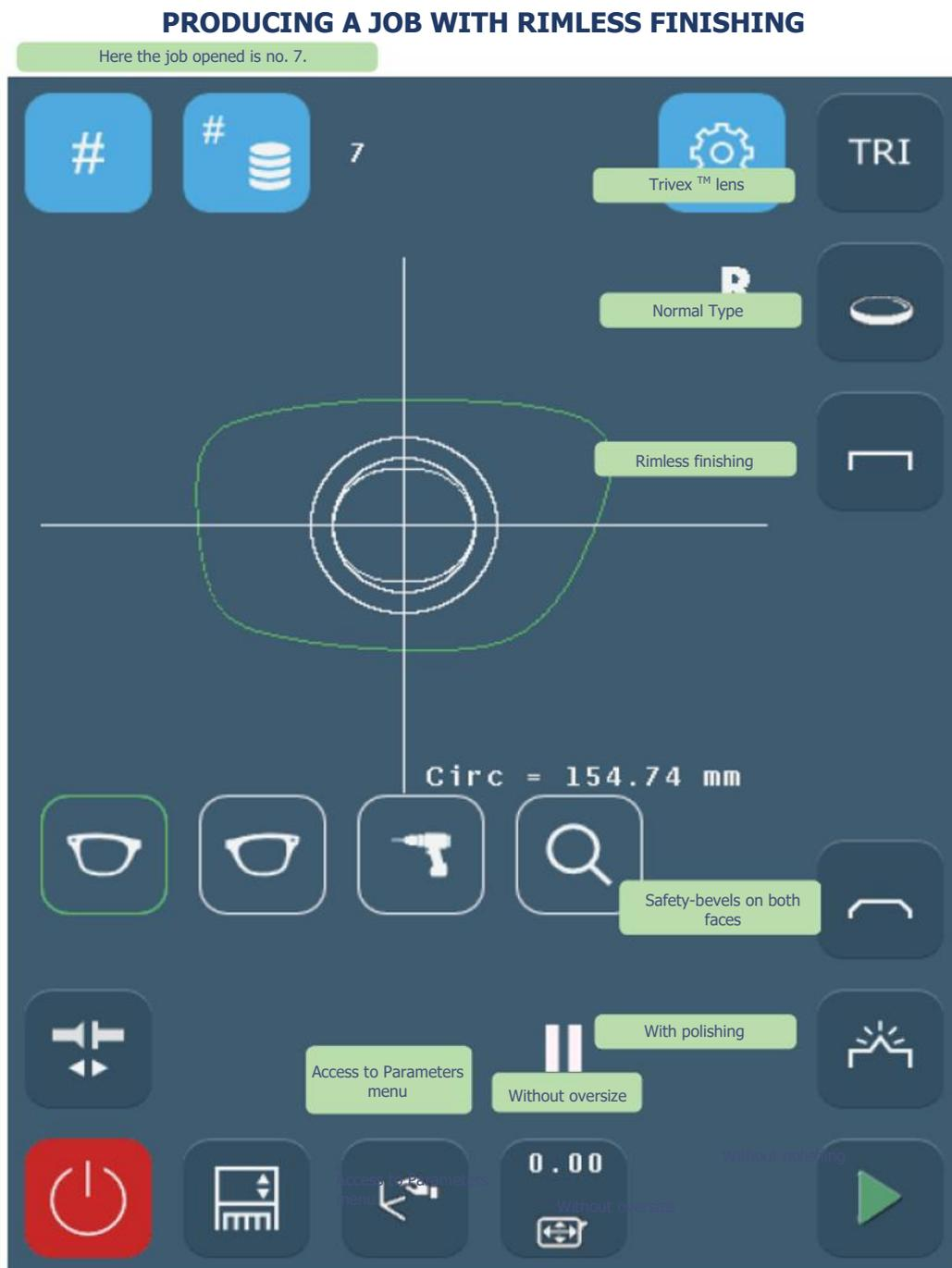
Screen 3-21: Example of the production of a job with rimless finishing
