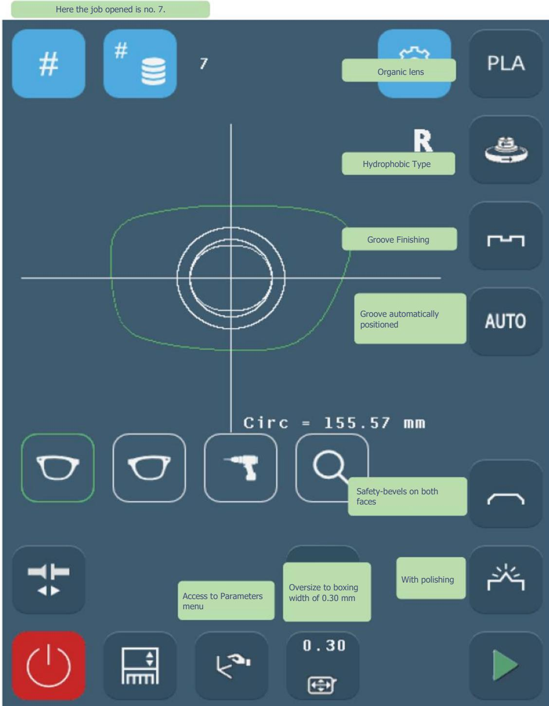
Screen 3-22: Example of the production of a job with a Groove
