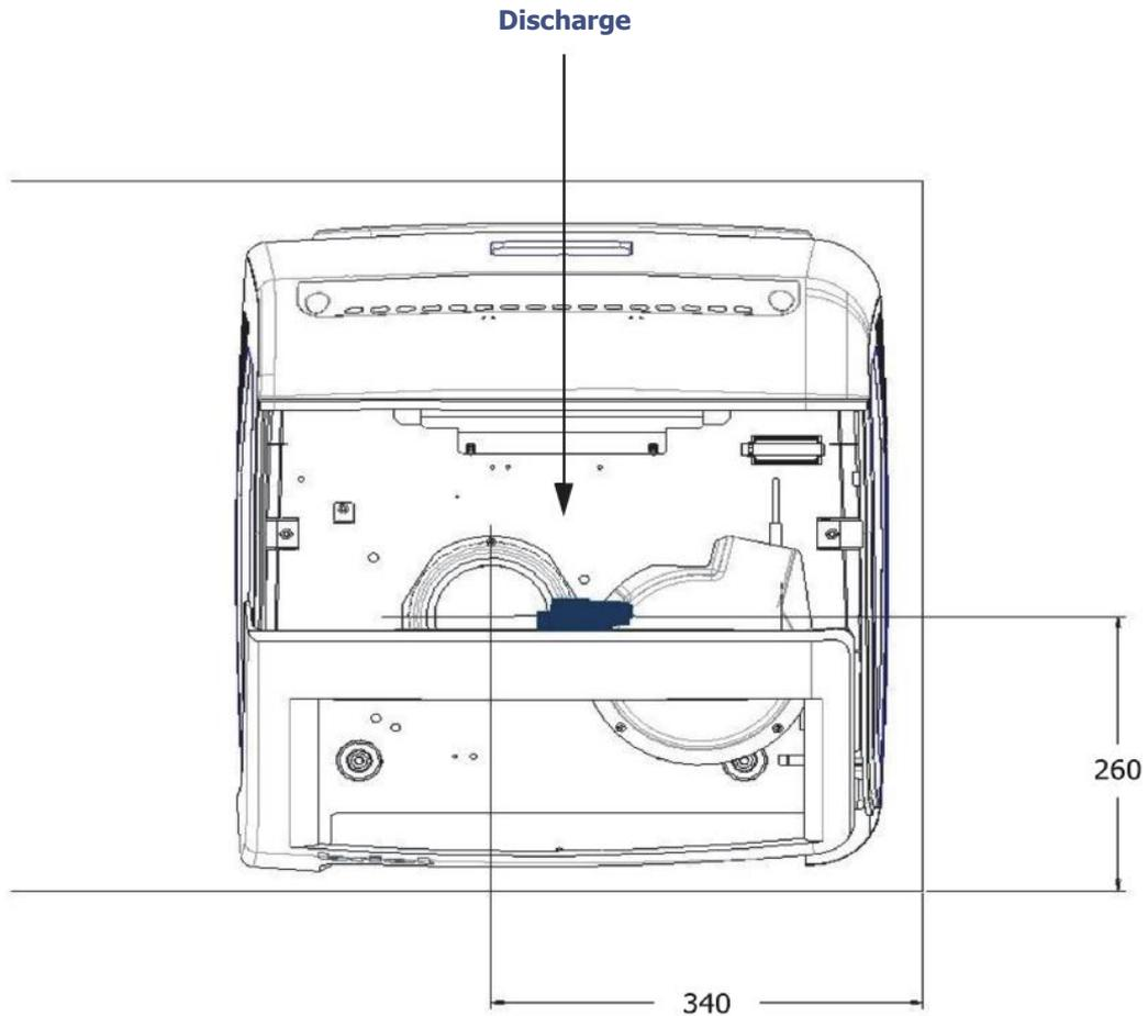
**Illustration 1-5 : Positioning the machine on the bench and drilling to be made**
