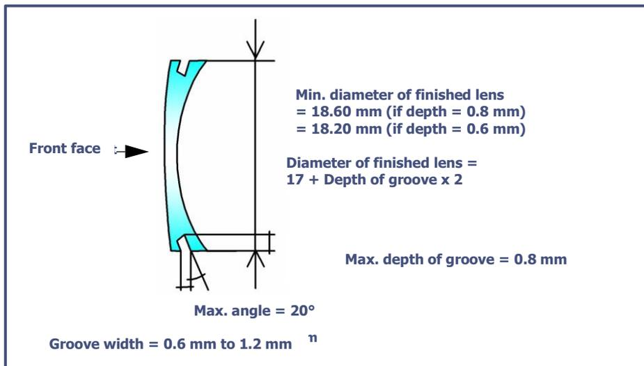
Illustration 3-6 : Limits of production of an inclined groove
