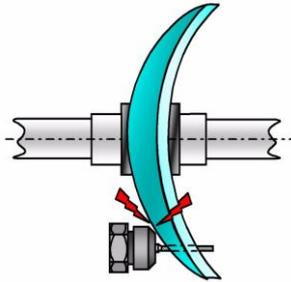
Example: Drilling 19 mm from the blocking centre at 0° in a lens of strength +7 D will produce a through hole.
