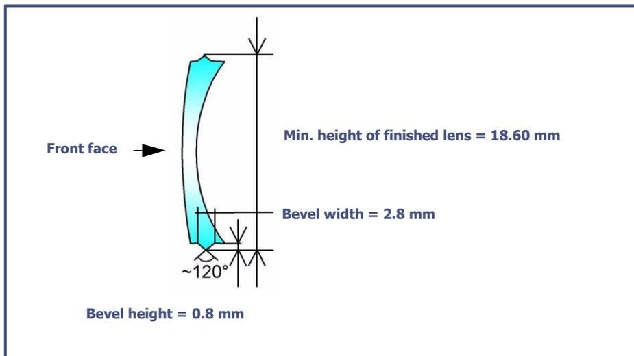
Illustration 3-4 : Limits of production of a bevel
