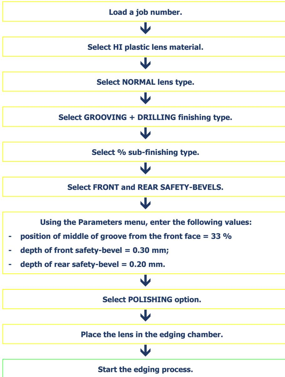
Flow chart 3-7: Production of a job with Drilling finishing
