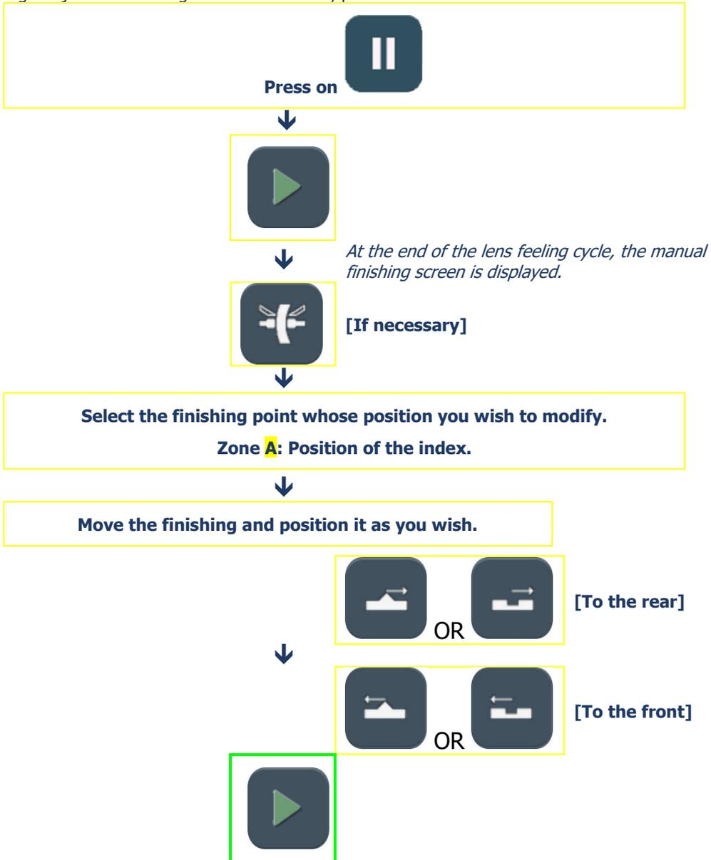
Flow chart 3-19: Placing a finishing manually
