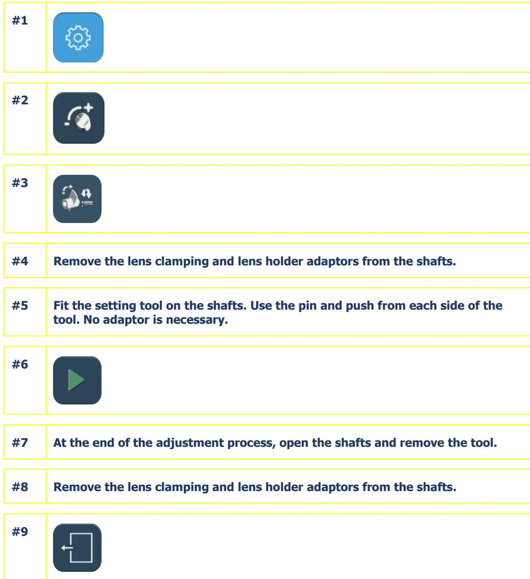
Flow chart 5-13: Adjustment of the axis setting with the tool
