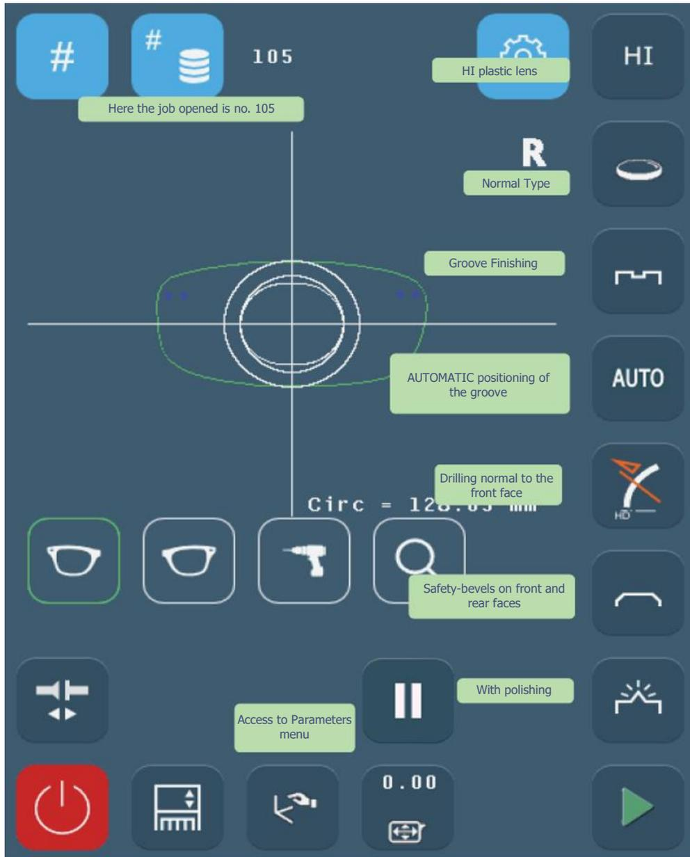
Screen 3-24: Example of the production of a job with Grooving and Drilling finishing
