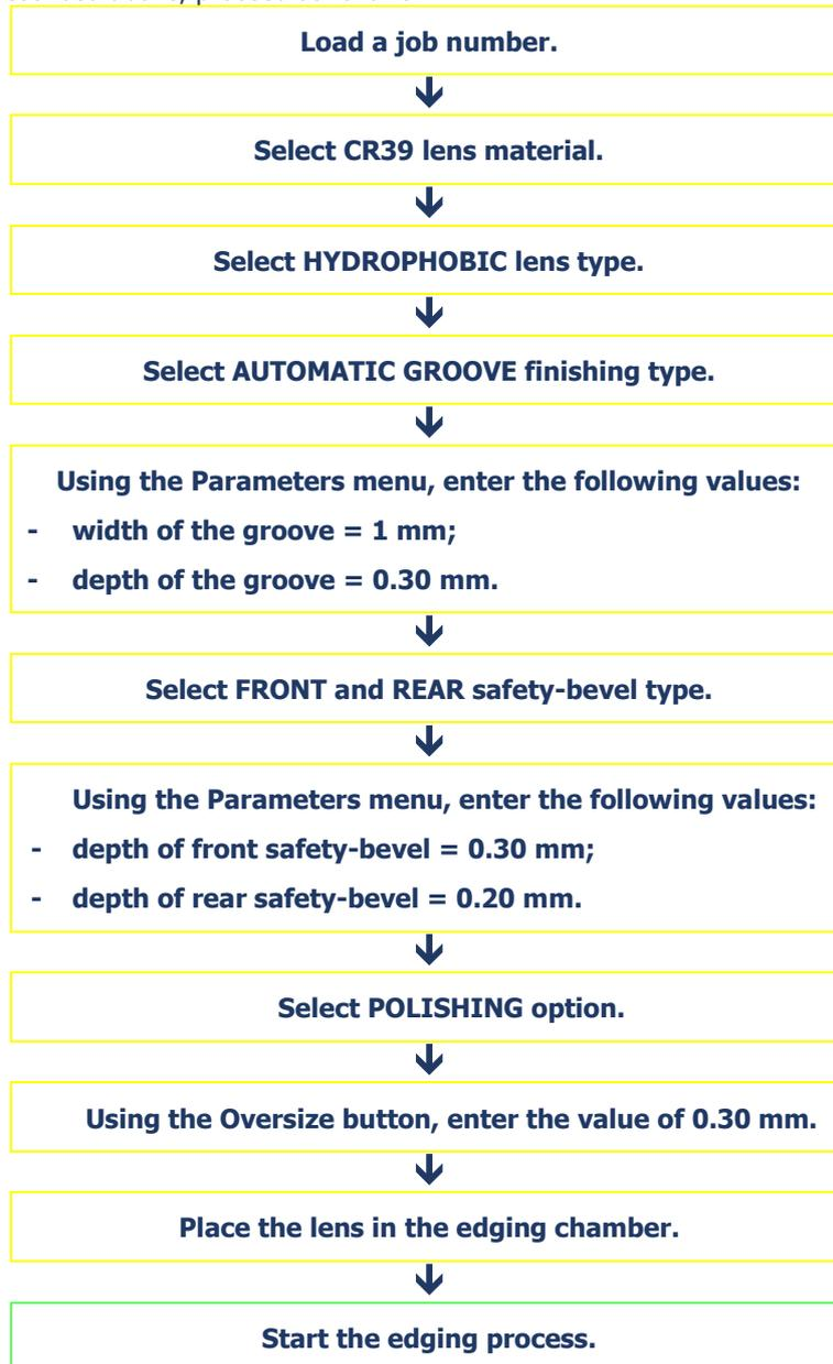
Flow chart 3-5: Production of a job with Groove finishing
