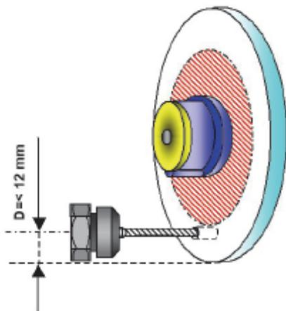
**Max. distance from drill bit centre - edge of lens = 12 mm**
