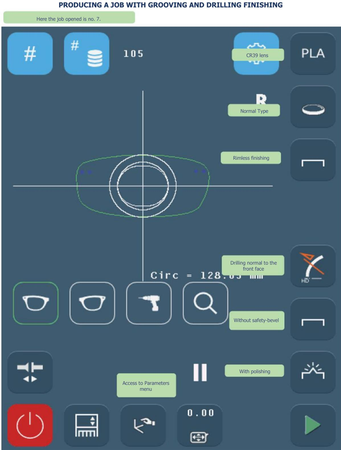
Screen 3-23: Example of the production of a job with drilling finishing
