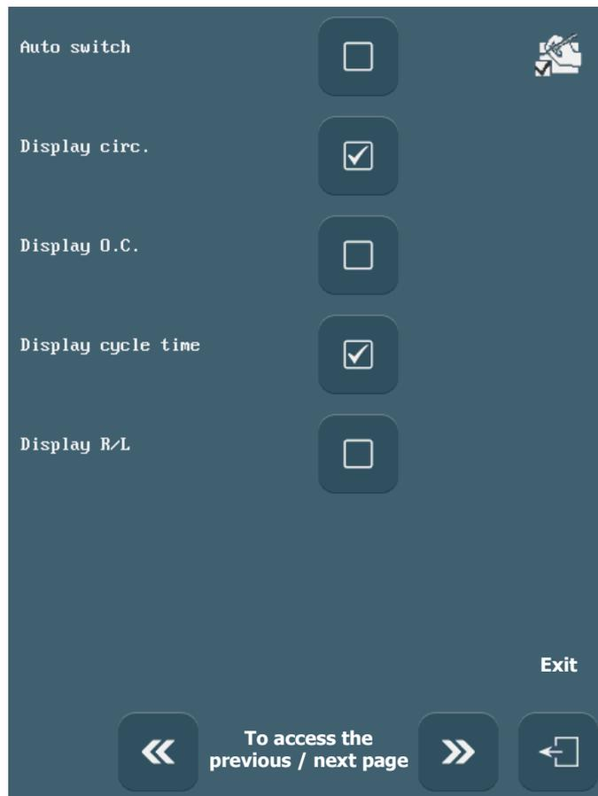
Screen 4-11: Setting the parameters of the machine's general operating functions (Page 4)
