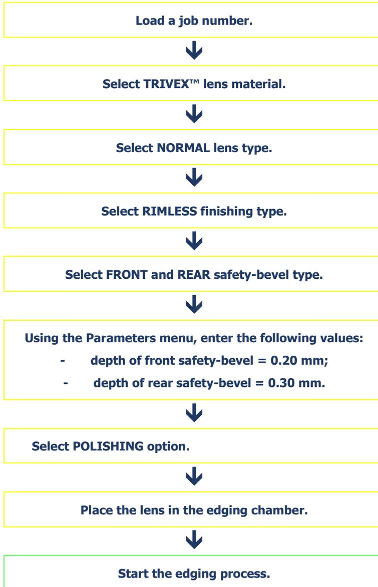
Flow chart 3-4: Production of a job with Rimless finishing
