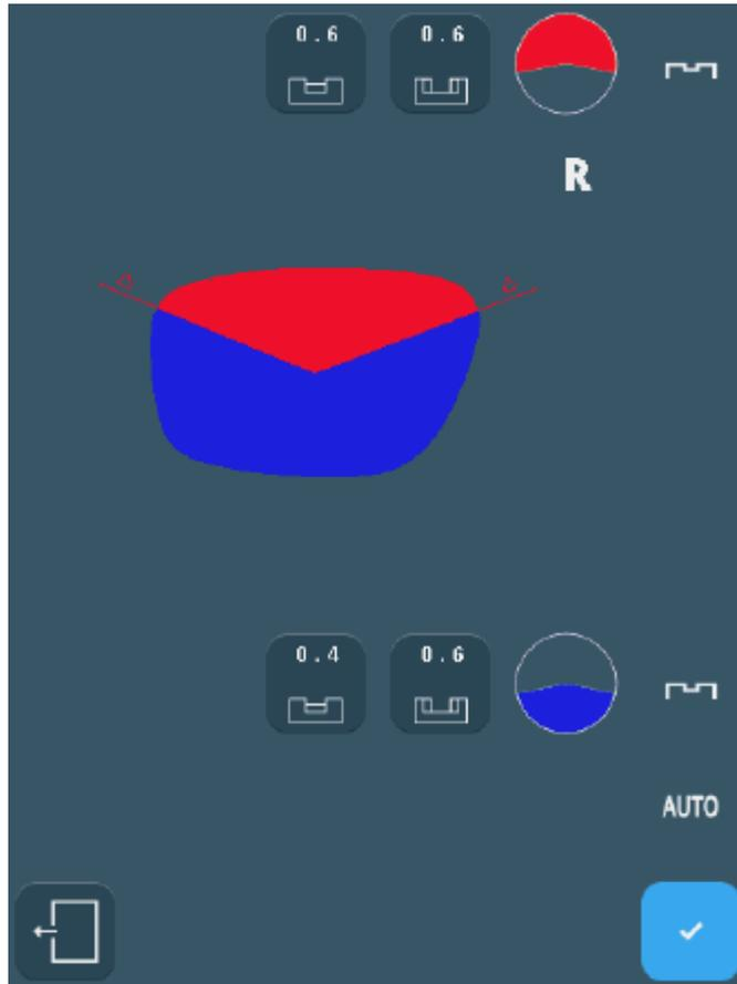
Note: If "Retouch" mode has been activated in the main menu, you can then increase the widths and depths of the grooves.
