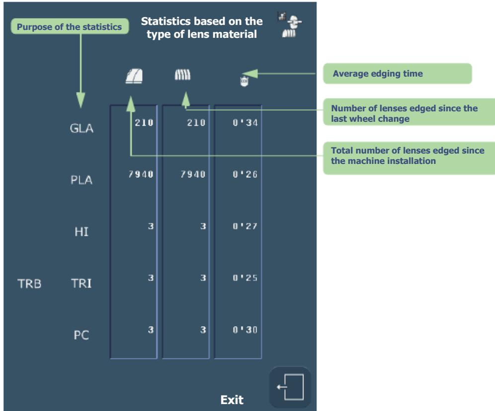
Screen 5-18: Display screen for statistics based on the type of lens material
