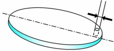
*Note: When the job is received on the edger, if it includes at least one hole whose diameter is smaller than that of the bit, the machine will display the following warning message: "Bit diameter > hole diameter. Do you want to drill?" If you reply Yes: the minimum diameter of the holes will be equal to the bit diameter. If you reply No: the entire drilling plan will be ignored and no hole will be drilled. The lens will be finished in rimless.*
