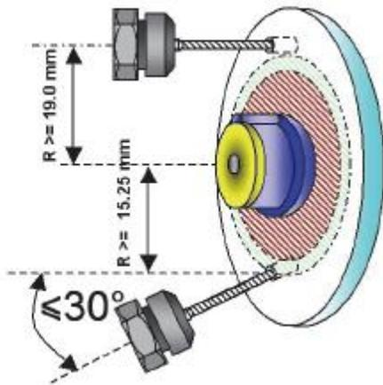
**Min. distance from centre of block - centre of hole = 19 mm (0°) or 15.25 (30°)**
