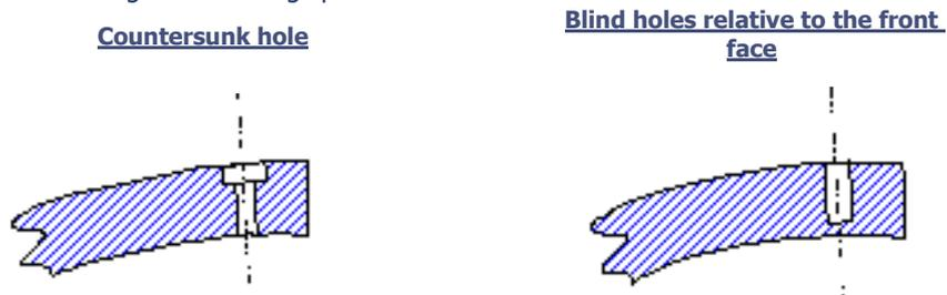
Countersinking is the superimposition of a blind hole over a through hole of smaller diameter.
