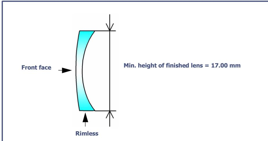
Illustration 3-3 : Limits of production of a rimless lens
