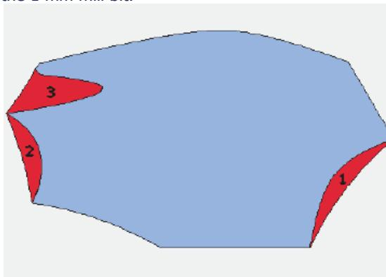
*Note: For shapes such as this where some areas are only machined with the 12 mm abrasive point (areas 1 and 2), all of the edge of the shape will be lightly finished using the abrasive point. In this case, polishing and safety beveling are not possible.*
