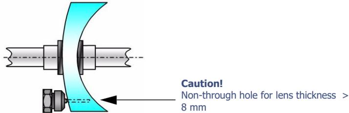
Example: Drilling 30 mm from the blocking centre at 0° in a lens of strength -7 D will produce a through hole.
