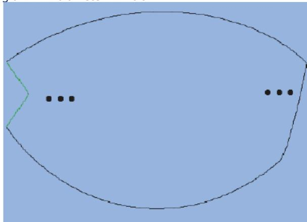
*Note:* For shapes such as this where the milled parts (shown in green) are produced using a 1 mm mill bit, polishing and safety beveling are possible. Finishing is carried out before cutting with the 1 mm mill bit (shown in green here).
