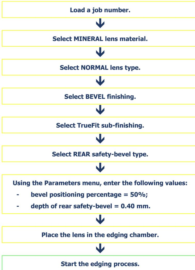
Flow chart 3-3: Production of a job with Bevel finishing
