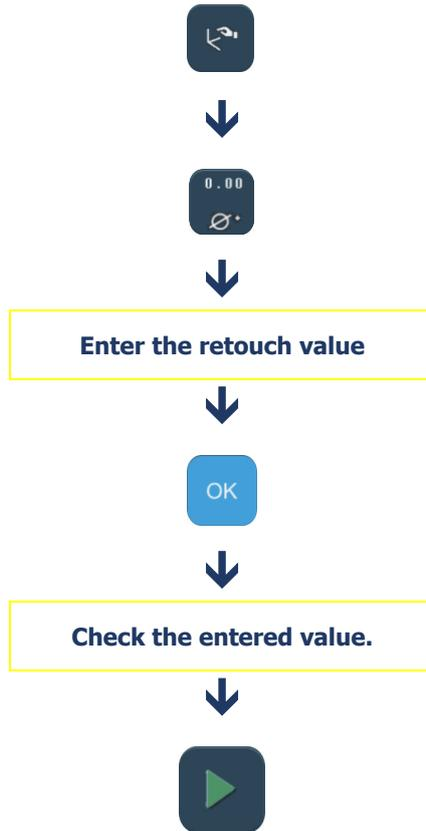
**Flow chart 3-11: rework of drilling identical for all the holes**
